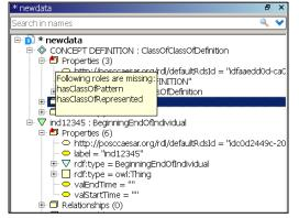
To create a new template instance open a view on a data source with template definition next to the panel with edited data source. Drag the required template and drop it on the root node of the edited data source. A form will appear indicating the template type and allowing entering the name of a new instance and URI – both optional. Template instances aren't usually assigned proper names.
