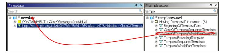
A type of an entity (Part 2 type or type of a template instance) can be changed by dropping new type (Part 2 or template definition respectively) on the *rdf:type* node in *Properties* node group of the entity. This can lead to exotic constructs (classes of individuals with relationship or template roles, relationships or templates with wrong role names, etc.) so the editor will try to determine wrong roles and warn you about them.
